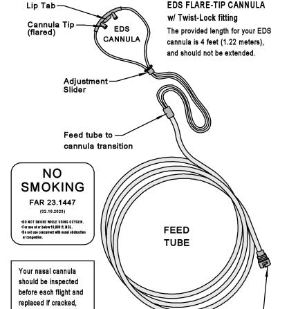
Bayonet Twist-Lock style fitting, for use
