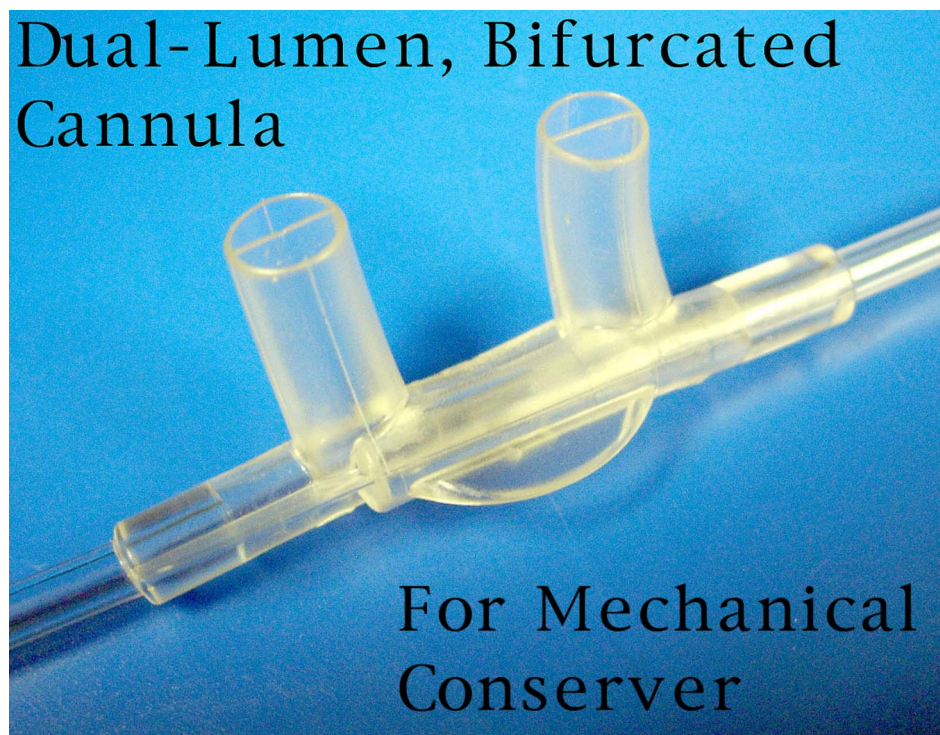
Figure 5. Dual Lumen Cannula. One tube acts as the inspiration (pressure) sensing line and the other delivers oxygen to the nose piece.
