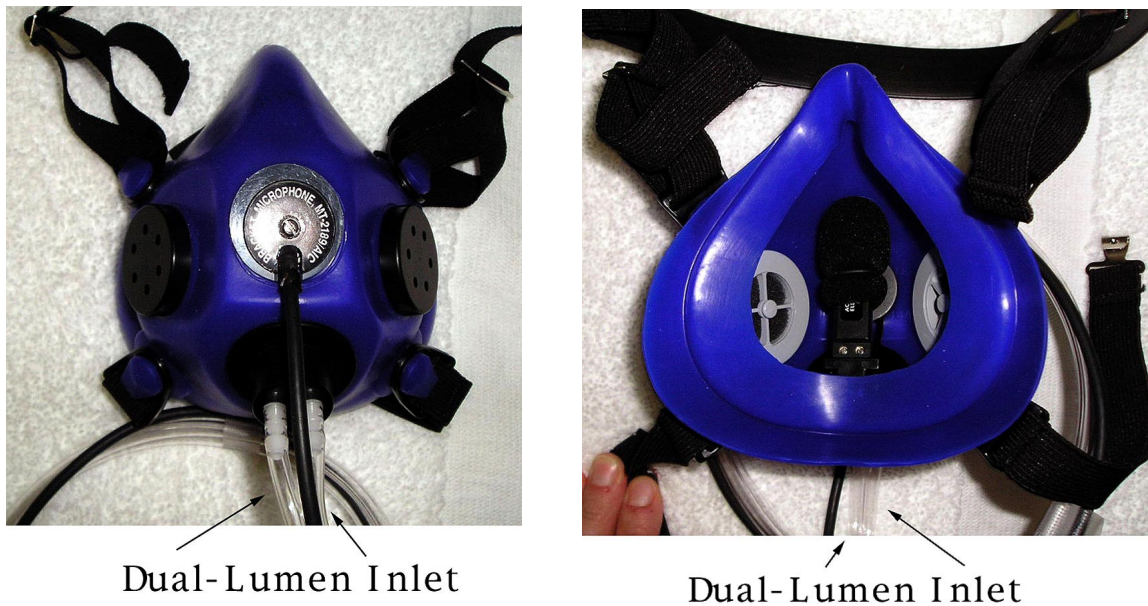
Figure 7. PF Deluxe Mask. Left photo shows the front of the mask with microphone connection at the nose of the mask, sensing/oxygen delivery line entering at the bottom of the mask and inhalation/exhalation valves at the side of the mask. Right photo shows the microphone center of the mask and the inside view of the inhalation/exhalation valves.
