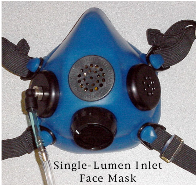
Figure 3. MH oro-nasal mask. The oxygen delivery pressure sensing line connects to the mask at the right cheek fitting. Mask features a voice transmitter (located at the nose of the mask) to propagate voice transmission through the mask and support use of a standard aircraft communication headset with boom-type microphone. A flapper-type exhalation valve is located at the lower center part of the mask, and an inhalation valve with flapper is located on the left cheek of the mask.
