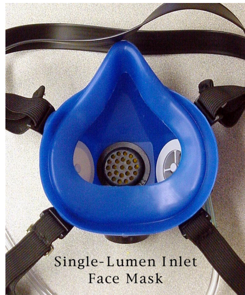
Figure 3. MH oro-nasal mask. The oxygen delivery pressure sensing line connects to the mask at the right cheek fitting. Mask features a voice transmitter (located at the nose of the mask) to propagate voice transmission through the mask and support use of a standard aircraft communication headset with boom-type microphone. A flapper-type exhalation valve is located at the lower center part of the mask, and an inhalation valve with flapper is located on the left cheek of the mask.
